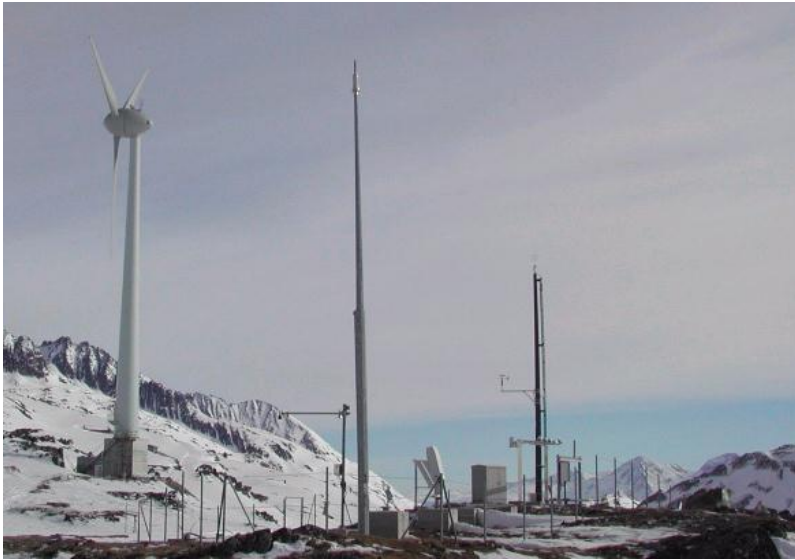
Figure 22. Installation on Mt. Gütsch with Enercon E-40 and test bench of the Swiss Met Institute.
