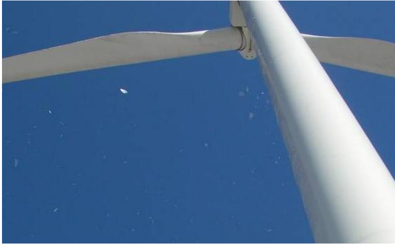
Figure 8-1: Ice falling or being thrown off a wind turbine poses a safety threat to turbine maintenance staff and, depending on turbine siting, the general public. Photo credit: Jeroen Van Dam, USA
